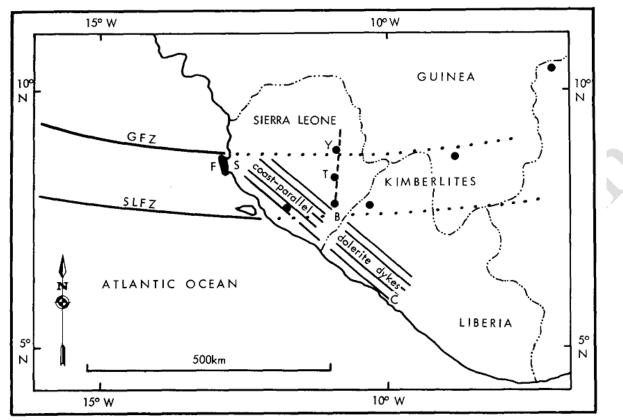
Fig. 3.2: Relationship between magmatism and regional structure in Sierra Leone and adjacent countries. B, Bagbe; C, Cape Mount; F, Freetown Complex; S, Songo; T, Tongo; Y, Yengema; GFZ, Guinea Fracture Zone; SLFZ, Sierra Leone Fracture Zone; solid circles, kimberlite; dotted lines, hypothetical continental continuations of fracture zones; dashed line, major fault controlling kimberlite magmatism [11].
